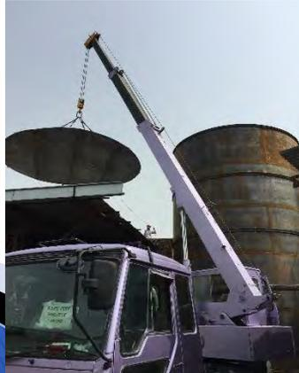
► **Manufacturing of 2 Nos. SS Milk Storage Tanks Dia 2760 x Shell Height 4000 x Thickness 6mm with 4 Nos, Legs Each.**
