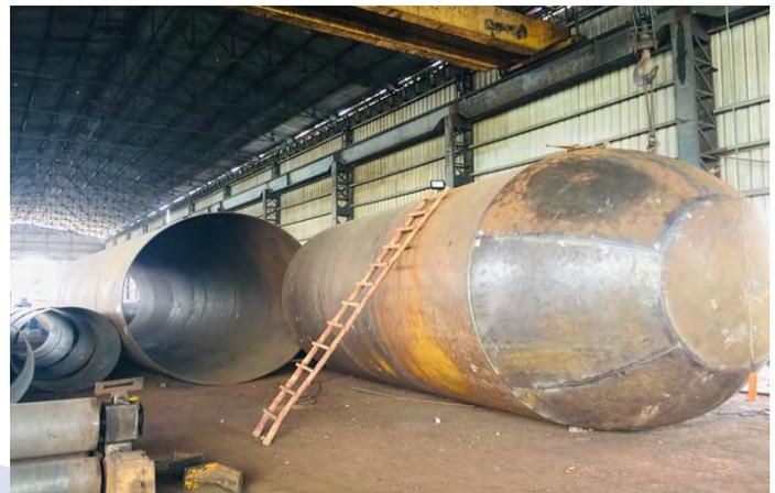
► **Complete Fabrication of 9 Nos. LPG Bowsers, Capacity = 30 MTONs each.**
